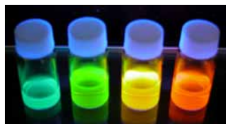
Emissive CdTe nanocrystals Quantum Efficiency >90%
